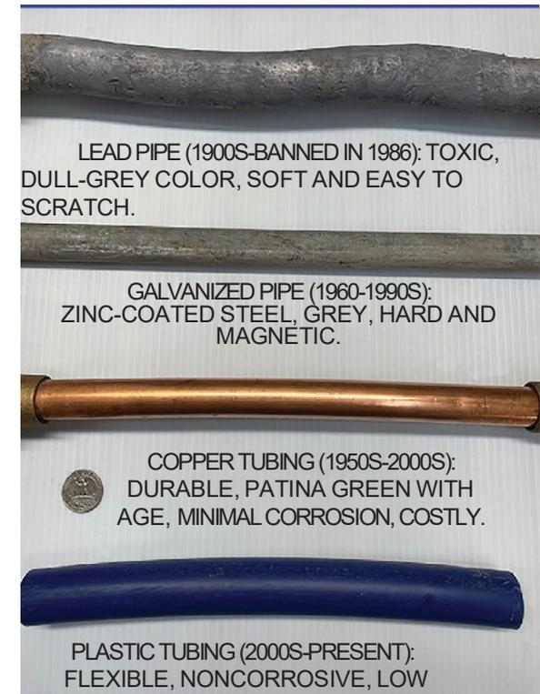
If you can't tell the difference between the steel and lead pipe, use a magnet- it will stick to the steel pipe but not lead.
